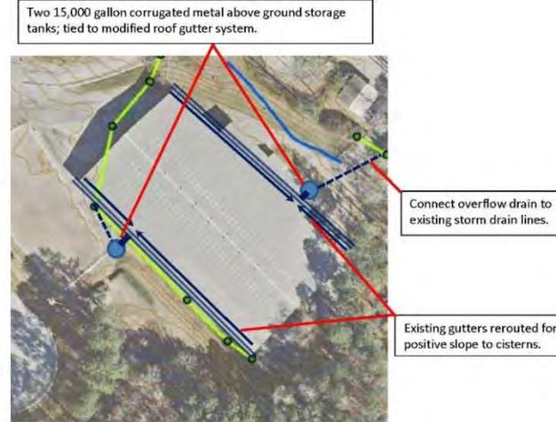
Plan view of water storage tanks and gutter system
