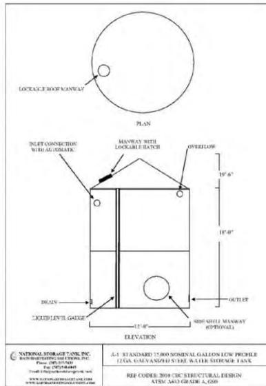
Schematic of a 15,000 gallon water storage tank
